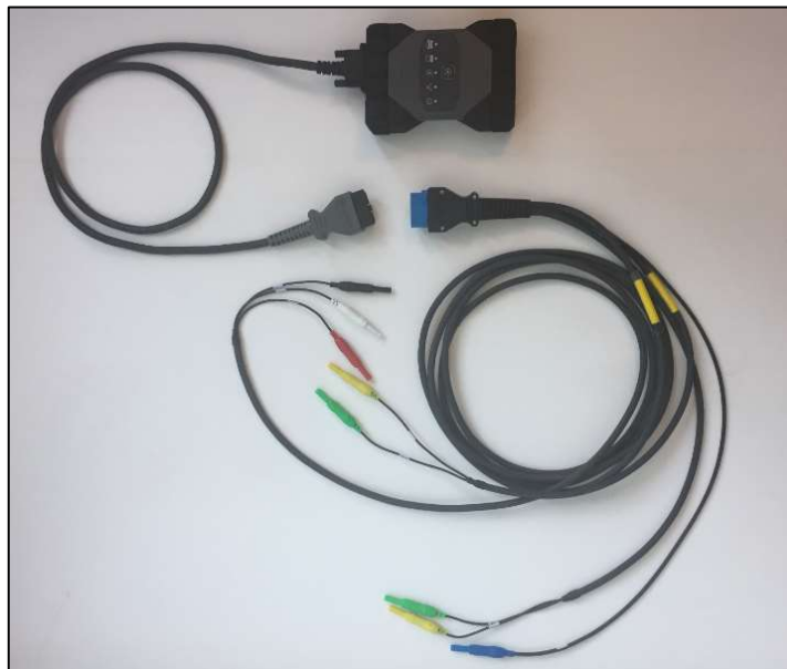
Image. 1: Measurement Cable OBD-Plug
