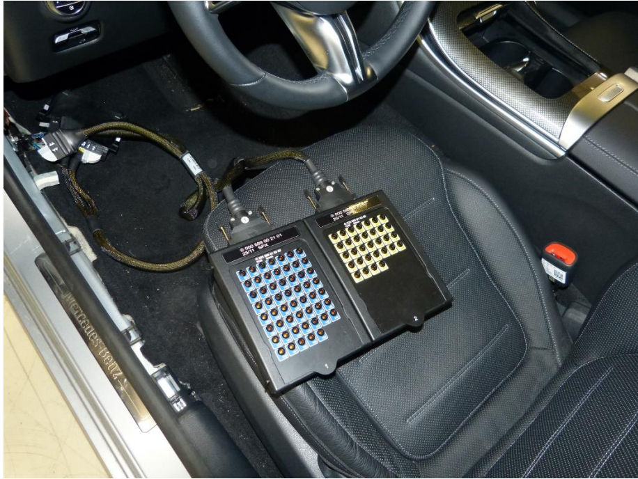
Image 3: Installation CAN-FD Model 206
