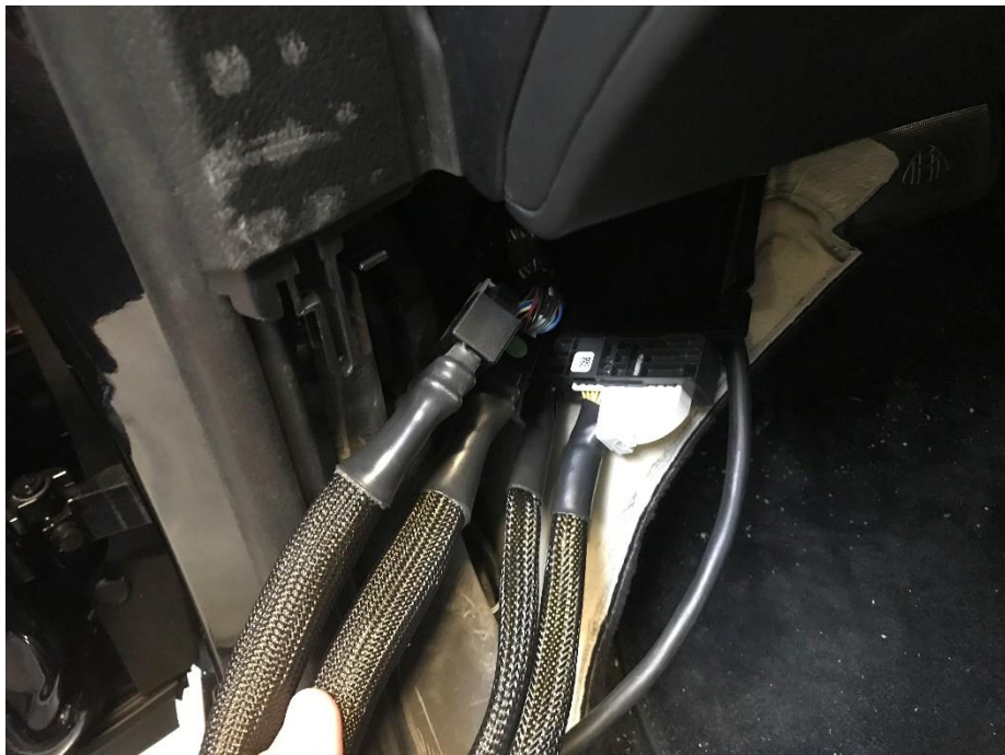
Image 4: Installation CAN-FD at CPC3 of Model 223
